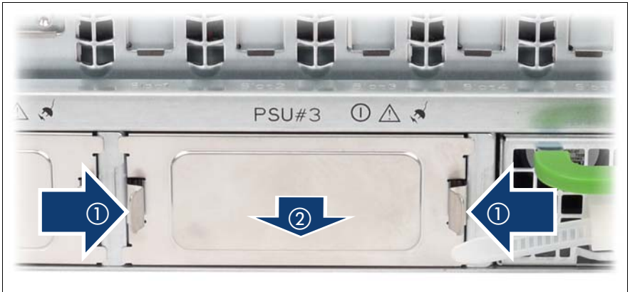
Figure 15: Removing a PSU dummy module
